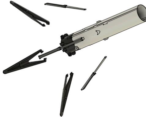
B. Attach all four landing legs and struts. Carefully twist in the struts to the pivot locations in the legs and body.
