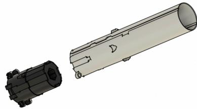
A. Glue the Engine Mount into the First Stage Bottom. Be sure to align the flat sides to match the raceway indents.
