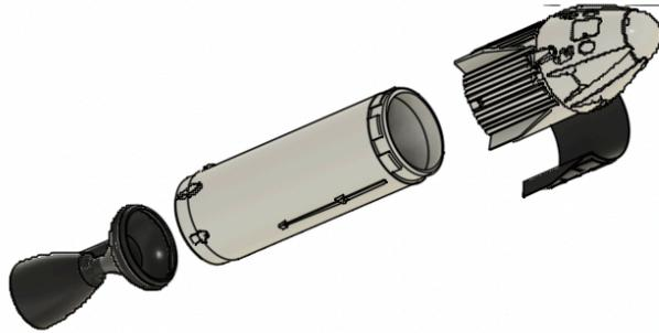
A. Glue the second stage engine into the second stage body.
