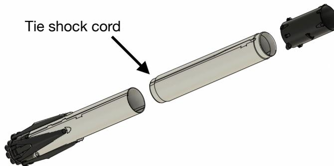
A. Glue the first stage halves and interstage together. Be sure to align the raceway indents and the launch lugs. Both lugs should be on the same side and same sized raceways should match.
