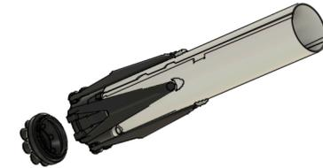
C. Fold the legs and screw in the engine cap.
