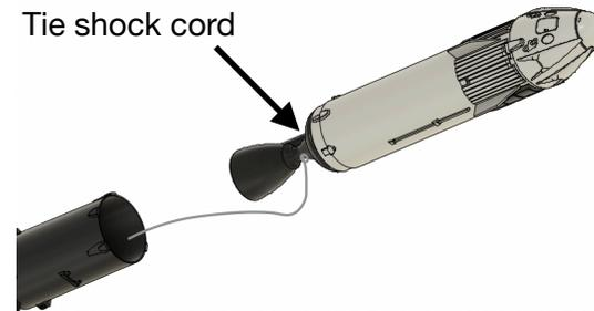
B. Tie the other end of the shock cord to the second stage engine, passing the shock cord through the gap in the engine.
