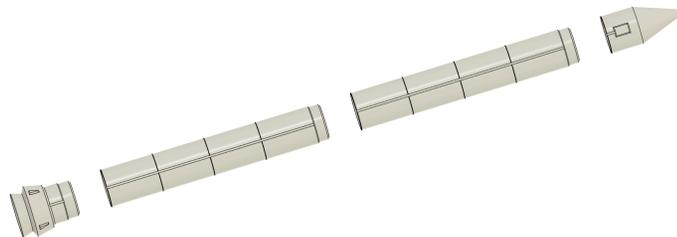
A. Glue the booster pieces together. Be sure to align the raceways. Do this for both boosters.
