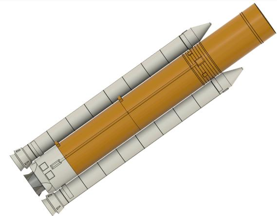
B. Glue the boosters into the SRB mounts on the core stage. Be sure to point the booster raceways away from the core stage. Level the booster engines with the core engines.
