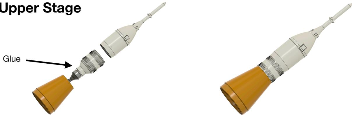
A. Glue the Interim Cryogenic Propulsion Stage (ICPS) Engine to the ICPS.
